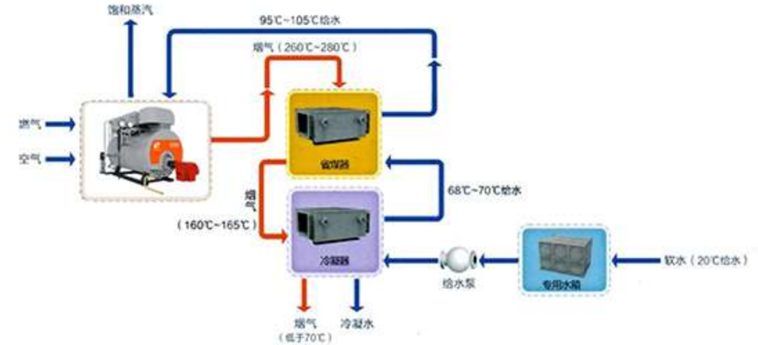
锅炉房系统图 Boiler Room System Diagram
